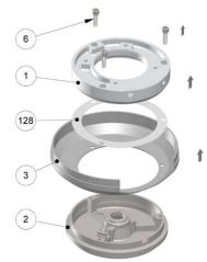
G - Turn the pump block over and remove the fixing screws (6). Separate the coupling flange (1), seal (128), eccentric part (3) and the cover (2).
