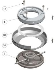
I - Remove the screws (11) and release the flange (5), the seal (128) and the eccentric part (30) from the cover (2).
