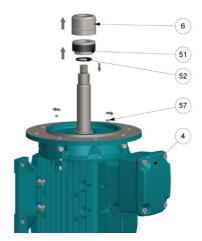
**M** - Loosen the fixing dowels on the rotating part of the mechanical seal (6) and remove it from the motor shaft (4). Remove the fixing dowels (57) from the bush (51) and remove it from the shaft and separate the O-ring (52).
