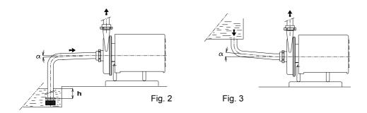
For this reason, when sucking from a tank located at a lower level, the pipe must reach below the free surface of the liquid. In order to prevent the formation of vortices and avoid the risk of sucking in air, always keep a minimum head at the pipe inlet (h. min.) equal to at least the dynamic head plus a safety margin of 0.1 m (Fig.2).
