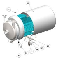
A - Remove the supporting feet (20-21-24-25-26-28) from the pump.
