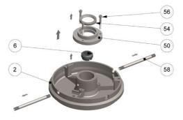
L - Remove the pipes (58) to flush the seal. Unscrew the screws (56), remove the radial mechanical seal (54) from the cover (50) and the fixed part of the mechanical seal (6) from the cover (2).
