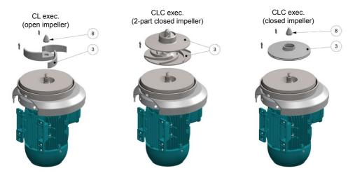
C - Use the relative wrench to loosen the impeller cover or the nut (8) and remove it by unscrewing anticlockwise.
