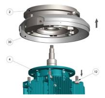
**H** - Unscrew the screws (12) and separate the pump unit from the motor (4).
