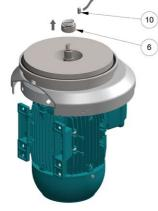
**D** - Remove the key (10) and the rotating part of the mechanical seal (6) inside the cover using two screwdrivers.
